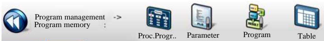
With this function, a program can be created or changed in the program memory of the controller. The operator is automatically guided to the necessary entries of the variable data. Phase-dependent basic settings such as monitoring, and safety functions are already stored for these program blocks in the system configuration and do not require any further processing. This eliminates incorrect entries and illogical constellations.
