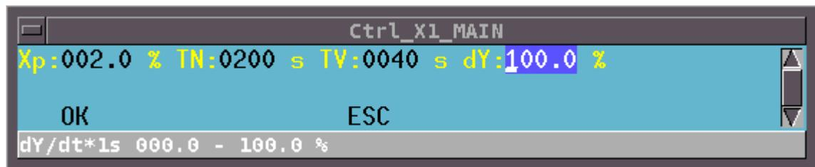
By means of the value "dY" the output of the controller block (the controller output) can be limited temporarily. In case of a jump of the setpoint, this effects that the controller output does not jump up but it adjusts itself slowly. The set value for "dY" causes a percentage changing of the controller output per second. Example:
